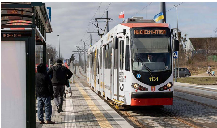
N8C-MF 01 1131 (Düwag, 1981) is seen on the new extension in Gdańsk along the street known as Warszawska on March 4. This car came from Dortmund, Germany in 2010. There it carried the number 131.
