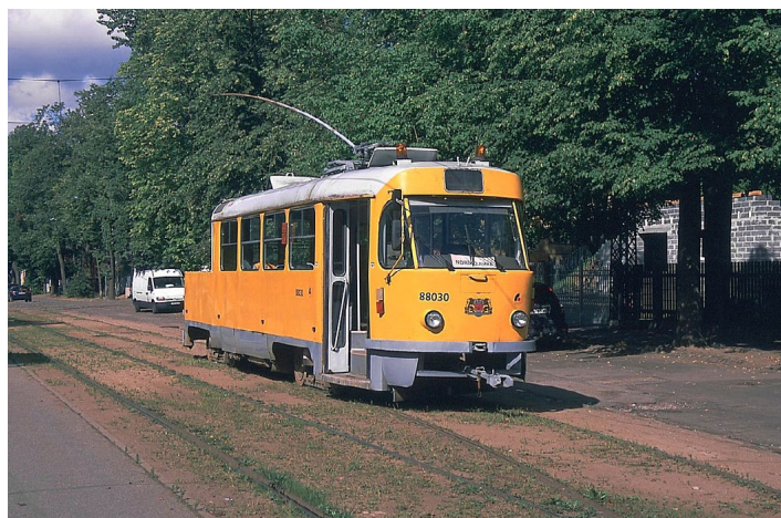
The roof over the rear end of a Tatra T3 PCC was removed to fabricate this work car for the movement of materials. How about some seats in that section to supplement car 1901 for good weather sightseeing?
