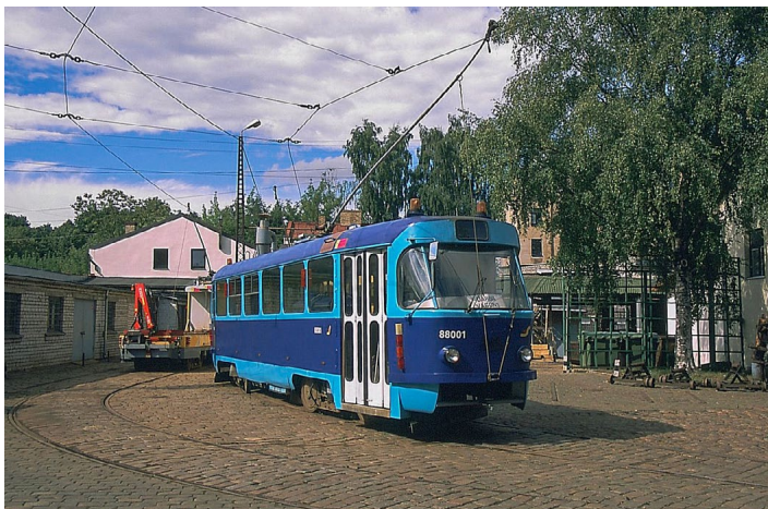
Rail grinder 88001 still looks like it could haul passengers. The two-tone blue livery is reminiscent of the color scheme used for New York City buses in the recent past.
