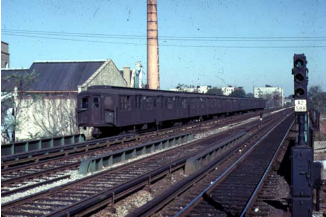
"A" motor 2651 entering the Avenue M station on the Brighton Line in November, 1961. 900 ABs were built from 1914 to 1922 (exactly 100 cars per year) plus 50 trailers in 1924. Originally built as single units, most were converted to 3-car "B" units. Some remained single units, and other combinations also were made. The ABs soldiered on until 1969.
