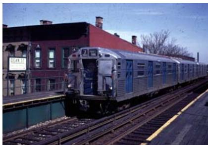
R-11 (R-34) 8011 at Dean Street on the Franklin Avenue Shuttle. In 1949, these stainless steel Budd-built cars were revolutionary. The R-11s, rebuilt as R-34s in 1964, spent their last days running on the Franklin Avenue Shuttle until 1976. One car (8013) survives in the Transit Museum.
