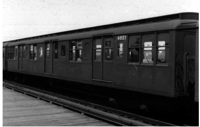
"BX" trailer 4021. These cars ran until the R-27s were delivered. Cars 4000-4044 ran as trailers in a 3-car set with cars from the 2400-2489 group on each end. Cars 4045-4049 had a Motorman's cab and were added to the ends of Canarsie trains during rush hours and were classified as "AX" units. In 1927, this practice ended and these cars became part of "BX" units with 2490-2499.
