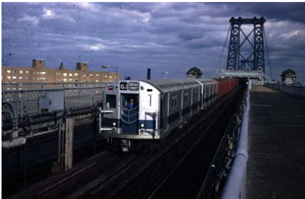
Multi-section 7017 on a July 22, 1961 fantrip on the Brighton Line. These high-speed (58 MPH on level track) lightweight cars, with their high rates of acceleration and braking, were an experience to ride. Over the years 1936 to 1961, these cars roared all over the BMT's Eastern Division, spending much of their time on the Canarsie Line and, during rush hours, heading out to Lefferts Avenue after branching off at Atlantic Avenue. None were saved from the scrapper.
