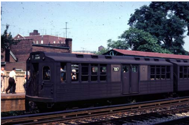
Multi-section 7017 on a July 22, 1961 fantrip on the Brighton Line. These high-speed (58 MPH on level track) lightweight cars, with their high rates of acceleration and braking, were an experience to ride. Over the years 1936 to 1961, these cars roared all over the BMT's Eastern Division, spending much of their time on the Canarsie Line and, during rush hours, heading out to Lefferts Avenue after branching off at Atlantic Avenue. None were saved from the scrapper.
