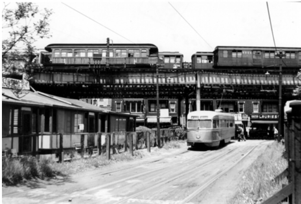
More of car 1083 in 1950, taken on the private right-of-way between Brighton Beach Avenue and Sea Breeze Avenue. Note the three types of BMT rapid transit equipment above the PCC — “Standard,” D-Type, and wooden elevated cars. Robert J. Wasche photograph
