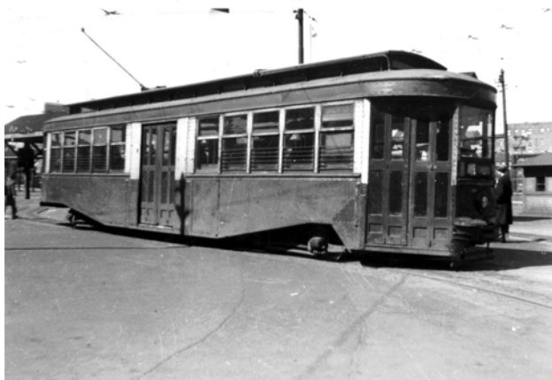
NYC Board of Transportation (ex-BMT) car 5108 at Williamsburg Bridge Plaza on April 7, 1946. The 5100-series cars were rebuilt for one-man operation. Bernard Linder photograph
