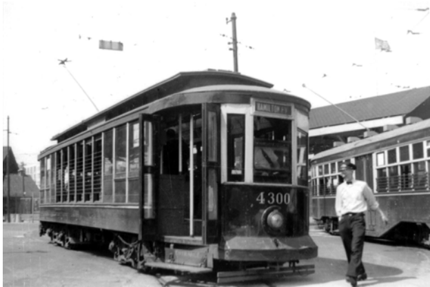
NYC Board of Transportation (ex-BMT) car 4300 at Williamsburg Bridge Plaza, August 30, 1941. 4100s and cars 4300-04 were rebuilt for one-man operation. Bernard Linder photograph
