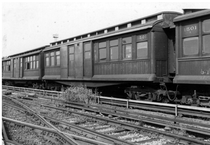
C-Type 1501 on September 13, 1955. Note that the doors are near the center of the car. This was changed on later units. Bernard Linder photograph
