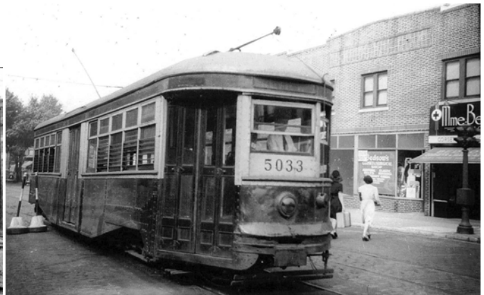
Car 5033, seen here on Flushing Avenue in Maspeth in 1944, was converted from double-ended/two-man operation to single-ended/one-man operation. Bernard Linder collection
