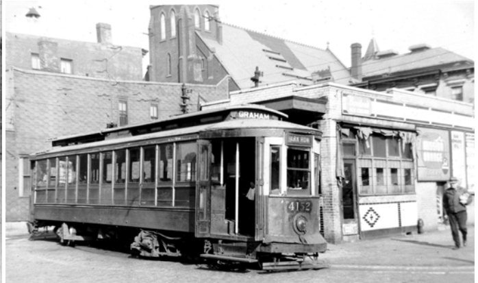
Long Island City Loop. Car 4152 was rebuilt from double-ended/two-man operation to single-ended/one-man operation. Bernard Linder collection
