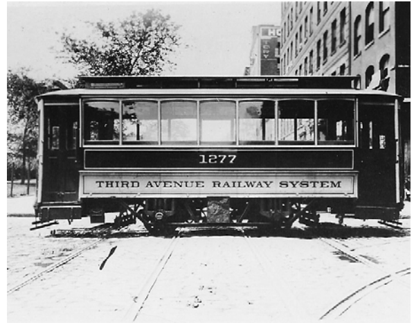
A Third Avenue Railway storage battery car on the 110th Street Crosstown Line. Bernard Linder collection
