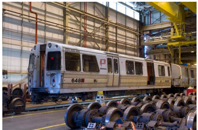
Car 648, a 1965 PA-1 from the St. Louis Car Company, sits with its front truck off during inspection.
