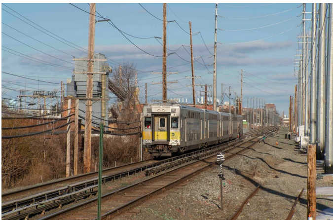
C3 5021 (Kawasaki Rail Car, 12/1998) is leading, with DM30AC 512 (EMD, 8/1999, s/n 956623-13) pushing from behind, Train #553 from Oyster Bay to Jamaica in this view east from the platform at the Merillon Avenue station on March 4. The new Nassau 1 Interlocking, with its Reduced Aspect signals, can be seen towards the rear of the train.
