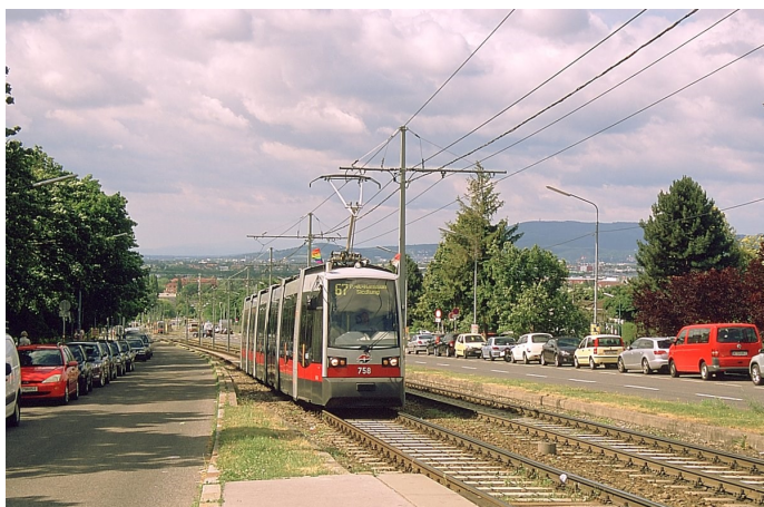
Type B1 758 (Siemens, 2013) is shown operating on Route 67 toward the city approaching the Sahulkastraße station. I stopped here to record the ballasted track on private right-of-way in the center of the road (Neulreichgasse), which is unusual for Vienna's system, which is dominated by street running shared with motor traffic. On September 1, 2019, Route 67 was replaced by Route 11.
