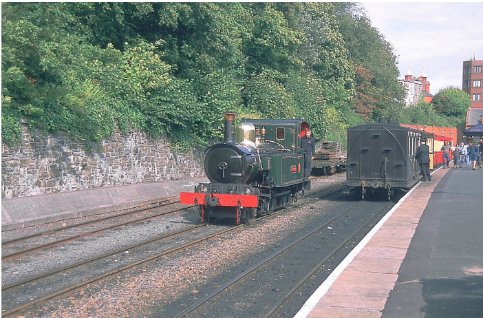
Locomotive 13, Kissack, is shown running around the train, but prior to coupling up it would be coaled and watered.
