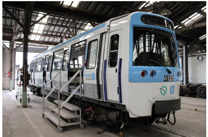
Paris Métro Line 8 MF77 train refurbishment. Jeremie Anne photo
