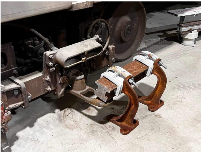
Demonstration W-S Standard Under-Running Third Rail donated by Metro-North at the Pennsylvania Trolley Museum.
