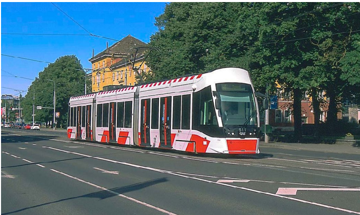
No. 511 is one of 20 CAF Urbos AXL trams built in 2015 for Tallinn. These single-ended three-section 100-percent low-floor articulated units were manufactured in Spain. A tender is being prepared for eight more modern low floor cars, with an options for as many as 20 more.
