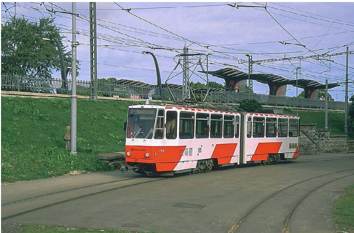
Tatra built this KT4 unit in 1986 for Erfurt. The PCC was one of 40 that came to Tallinn between 2006 and 2013. Prior to being placed into service these cars were regauged from one meter to 3 feet 6 inches (1.067 meters), following in the footsteps of others (now retired) also obtained from various East German tramways. A low-floor center section was added to 12 of these KT4s (which became KT6Ts) between 2004 and 2007, but all have since been retired.
