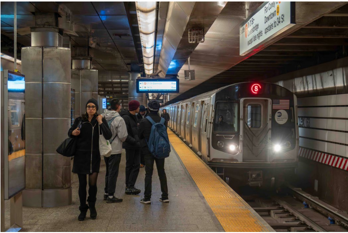
The 1720 F from 21 Street has arrived at Lexington Avenue, discharged most of its passengers and is now continuing south to just beyond the Lexington Avenue Interlocking before changing direction and heading back to Queens on the late afternoon of March 21. R-160A-1 8529 (Alstom, 4/2008) led the eight-car consist. The F shuttles were signed up as S shuttle trains. Jeff Erlitz photo
