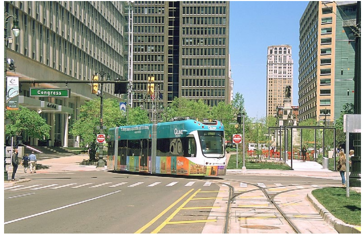
(Above and below) Two views at Congress Street, the southern end of the line. The upper photo shows a car about to pull into the terminal stop, while the lower shows it laying over while its batteries are being charged. No. 292 will soon pull out and take the curve to the right. I suspect the special work shown above is a spring switch. In the background is Campus Martius Park, which is circumscribed by the line. Both roadways carry the Woodward Avenue designation.
