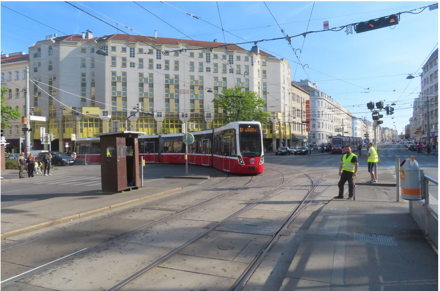
Type D No. 339 (Bombardier Transportation, 12/2022) is turning off Quellenstraße and onto Laxenburger Strasse, at Quellenplatz, on another piece of normally non-revenue trackage. This is currently Vienna’s only \frac{3}{4} Grand Union (Vienna never had a complete one). The switchmen here set rarely used switch points that are not electrified. An interesting feature here is the sign “X” on the wires above (next to the signal) with an arrow pointing to the left. This means a ban on meeting in the bend due to clearance issues. Once upon a time, there were many “XZ” signs around the system. The Type Zs were the former Third Avenue Railway cars from New York. Due to their considerably greater width than the normal Viennese cars, there were often bans on meeting in curves.
