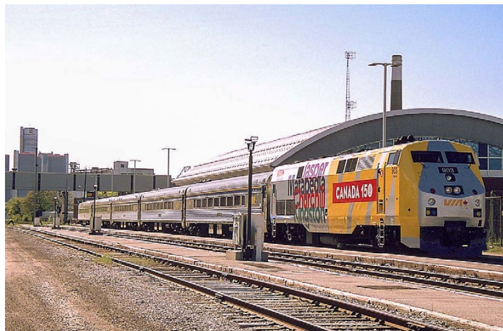
A scene at the railway station in Windsor. (If you say Windsor Station, everyone thinks you're talking about Montreal.) This is Via No. 78, the 5:45 p.m. corridor train to Toronto with a General Electric-built P42DC at the point. The Genesis unit was built in 2001 and was one of the last of its type to be manufactured. It is bedecked in the special 150th anniversary color scheme and markings that commemorate the creation of Canada in 1867. The five fluted-steel passenger cars are loading passengers from the platform adjacent to the station building. Built by the Budd Company in the 1950s for several American roads, Via Rail obtained the cars from Amtrak and then had them rebuilt in the 1990s. One of the units is a club car, providing first class service including hot dinners.
