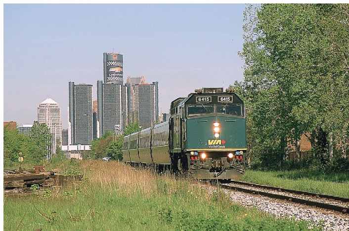
Via train No. 72, from the George Avenue grade crossing in Windsor just after it started its journey at 9:05 a.m. No. 6415 is an F40 built by General Motors in 1987. The rolling stock consists of Bombardier-built LRC (light, rapid, comfortable) coaches (and a club car) built in the 1980s. When they first went into service, these cars ran with matching locomotives, but those wore out by 2001 and were scrapped. This photo was taken with a zoom lens. Prominently in the background is the world headquarters of General Motors in the Renaissance Center, located on the other side of the Detroit River. If Dinah Shore were standing next to me she might have reversed the old iconic slogan as: See a Chevrolet in the U. S. A. . . . https://www.youtube.com/watch?v=CX3MaOJTtsc
