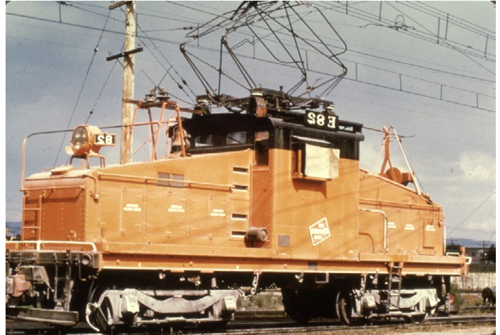
Milwaukee Road Steeplecab switcher #E-82, class ES-2 (Alco-GE, 1917). This would later become the last Milwaukee Road electric to operate. Date, location and photographer unknown, ERA collection.
