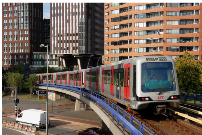
An example of Rotterdam's oldest current metro cars, Type MG2/1 No. 5341 (Bombardier Transportation, 1998–2001) leads a train about to enter the Rijnhaven station on Line E on August 29, 2019. Frantisek Vanasek photo via Urban Electric Transit
