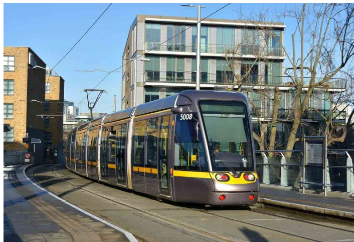
Citadis 502 No. 5008 (Alstom, 2009) is at the Charlemont stop of the Green route on January 10, 2026. This car had been converted from a Citadis 402 in February 2020. Zxs91 photo via Urban Electric Transit
