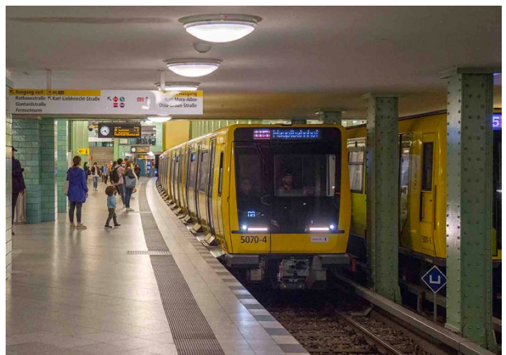
Type IK20 No. 5070 (Stadler, 7/2020) shows the plates mounted at the bottom of the doors to enable operation on Line U5. Alexanderplatz Station on September 22, 2022. Jeff Erlitz photo
