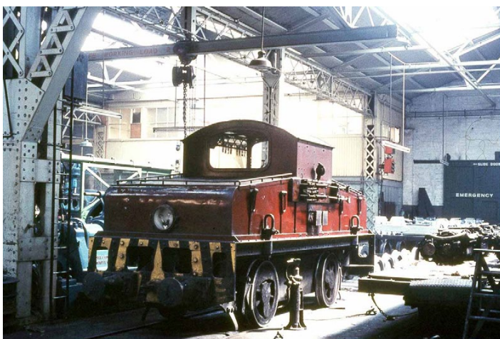
Glasgow Subway battery locomotive No. 1 at the Govan Cross Workshop.
