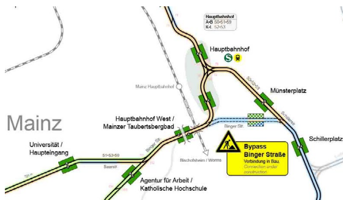
Detail of tramway track diagram of Mainz, showing the new bypass on Binger Straße. Christian Stade/gleisplanweb.eu
