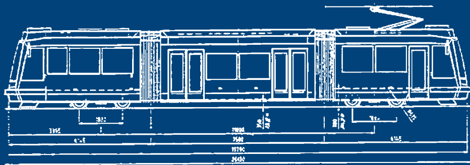
Streetcar Elevation. 20 meter (66') length.
