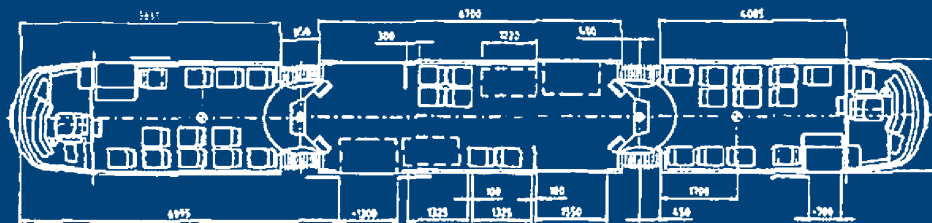
Streetcar Floor Plan. 2.46 meter (8') width.
